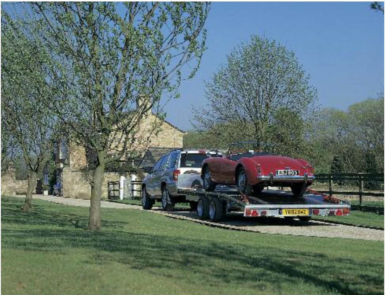
LM167/B with optional headboard skids, electric winch, propstands & lashing rings
